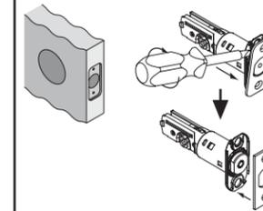
Chisel 1/8" (3 mm) deep or until latch face plate is flush with door edge.
