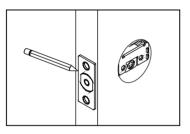
Insert latch in hole, mark outline of faceplate and remove latch.
