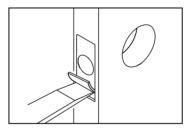
Chisel 1/8" (3mm) deep or until faceplate flush with door edge.
