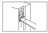
Measure one half of door thickness from door stop and vertically mark center line of strike. Drill aperture which is same with strike box 1-9/64" (29mm) deep at inter section of horizontal and vertical center line of strike. Match screw hole on strike with center lines on jamb. Mark outline and chisel 9/32" (7mm) deep for strike.
